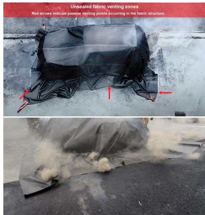
Figure No. 1: Passive airflow; no sealed edges transform the fire from a “sealed bomb” to a controlled pressure system.
